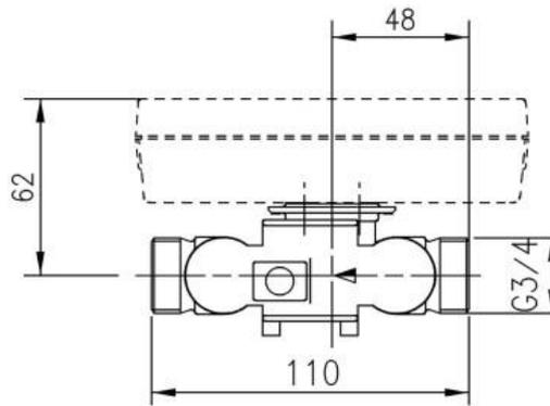
Fig. 1: Overview dimensions overall length 110 mm (thread)
