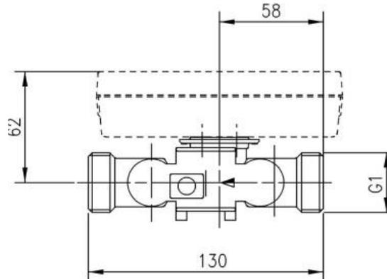
Fig. 2: Overview dimensions overall length 130 mm (thread)
