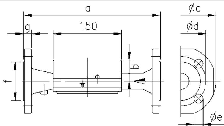
Fig. 7: Overview dimensions of large meters with flange
