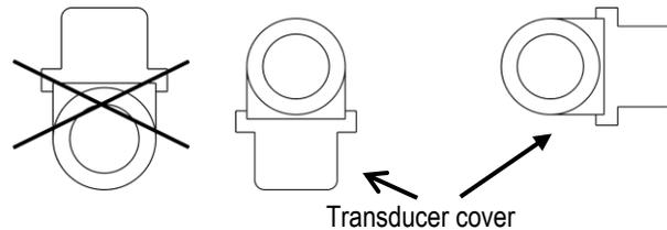
Fig. 14: Recommended installation position for cooling metering
