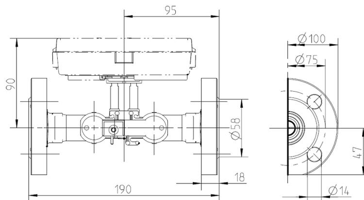
Fig: Overview dimensions overall length 190 mm (flange)
