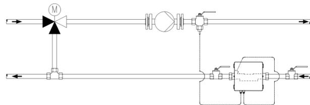
Fig. 11: Installation for circulation with admixing; placement of temperature sensors
