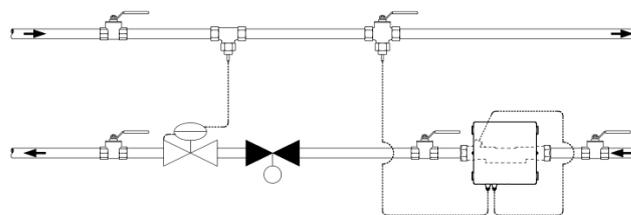
Fig. 12: Installation for circulation with throttling configuration for example (flow sensor in flow direction upstream control valve / differential pressure regulating valve)
