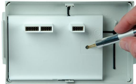
The contact pads must be shorted while the calculator top is still active (display on). If it is not possible to keep the calculator top active, the recommendation is to remove the communication modules from the base, assemble the calculator and then open the calculator again and short the contact pads.
