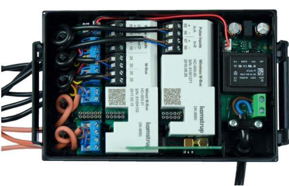
Wireless M-Bus-module with internal antenna
