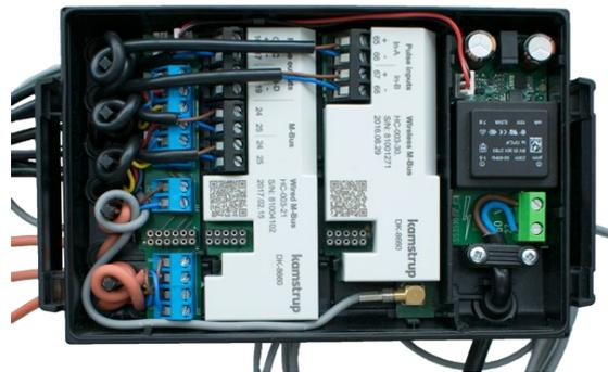
Wireless M-Bus-module with external antenna
