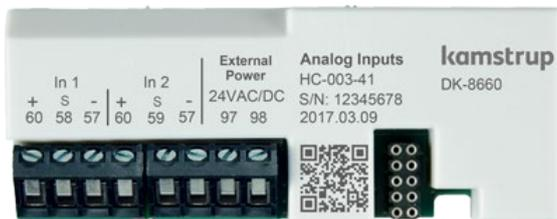
The external 24 VAC/DC supply is used to supply the analog input circuit and the attached sensors.
