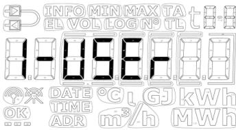
"USER loop" is the meter's primary loop, which includes legal and mostly used readings. The loop is intended for the user and is configured according to the user's requirements via the DDD-code. See paragraph 3.2.4 for further information on "USER loop" and DDD-codes.
