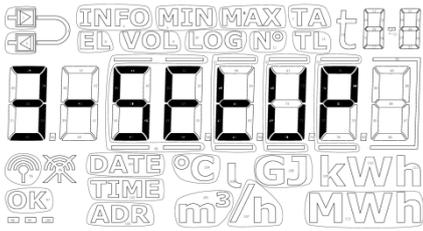
In this loop the technician can configure the meter via the front keys. This enables the technician to configure the meter both before installation and after commissioning of the meter. Configuration of the meter after commissioning requires that the installation seal is broken and that meter top is separated from meter base.
