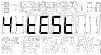
"TEST loop" is used by authorized laboratories for reverification of the meter among other things.
