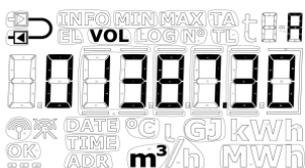
**16. + 17 Meter numbers of Inputs A and B**
