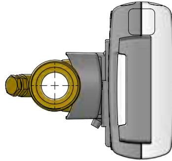
**Note:** In case of compact mounting, it may be necessary to use the enclosed angle fitting with some types of ULTRAFLOW® to obtain the required combination of viewing angle for the calculator's display and installation angle for ULTRAFLOW®.
