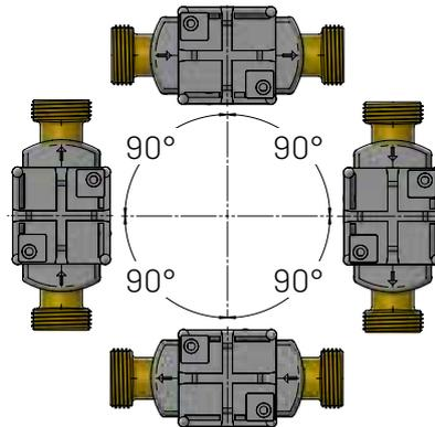
The flow sensor can be mounted horizontally, vertically or at an angle.
