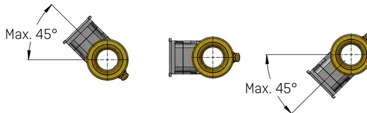
The flow sensor should be mounted with the plastic casing placed on the side [at horizontal mounting].
