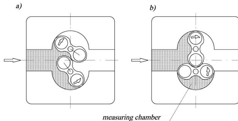
Fig. 2. Operation of the rotary gas meter.
