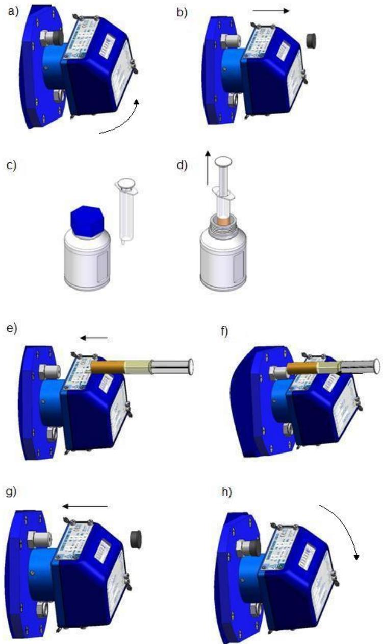
Fig. 18. Oil refill procedure in pressurized conditions.
