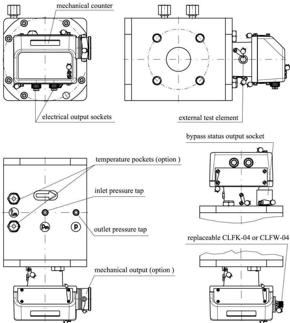
Fig. 4. Location of measurement outputs of the CGR-FX gas meters.
