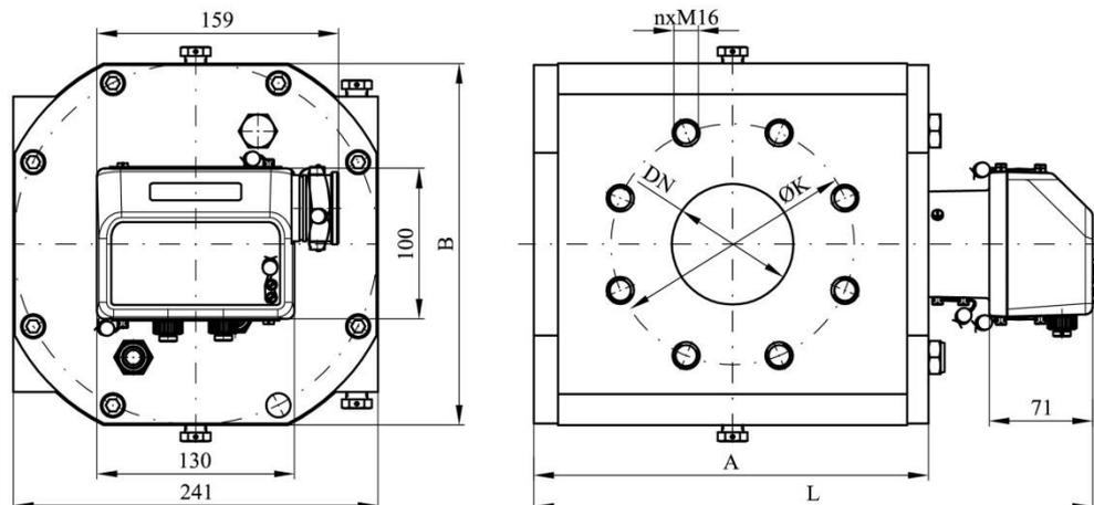
Fig. 14. Basic dimensions of CGR-FX rotary gas meters.
