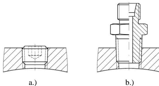
Fig. 6. 1/4" NPT pressure measurement tap
