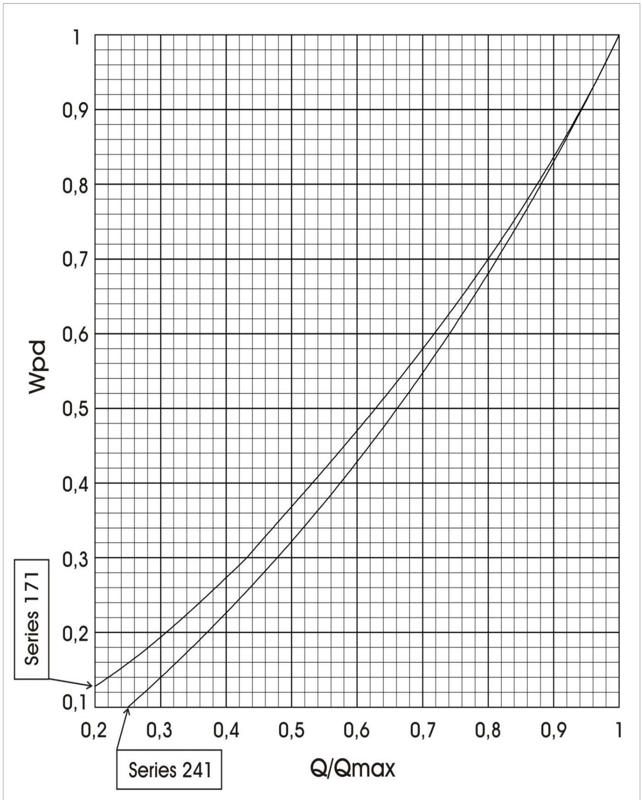
Fig. 1. Pressure drop coefficient as a function of the relative flow  $Q/Q_{max}$ .
