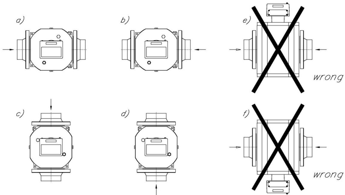
Fig. 12. Operating positions of the CGR-FX rotary gas meter.
