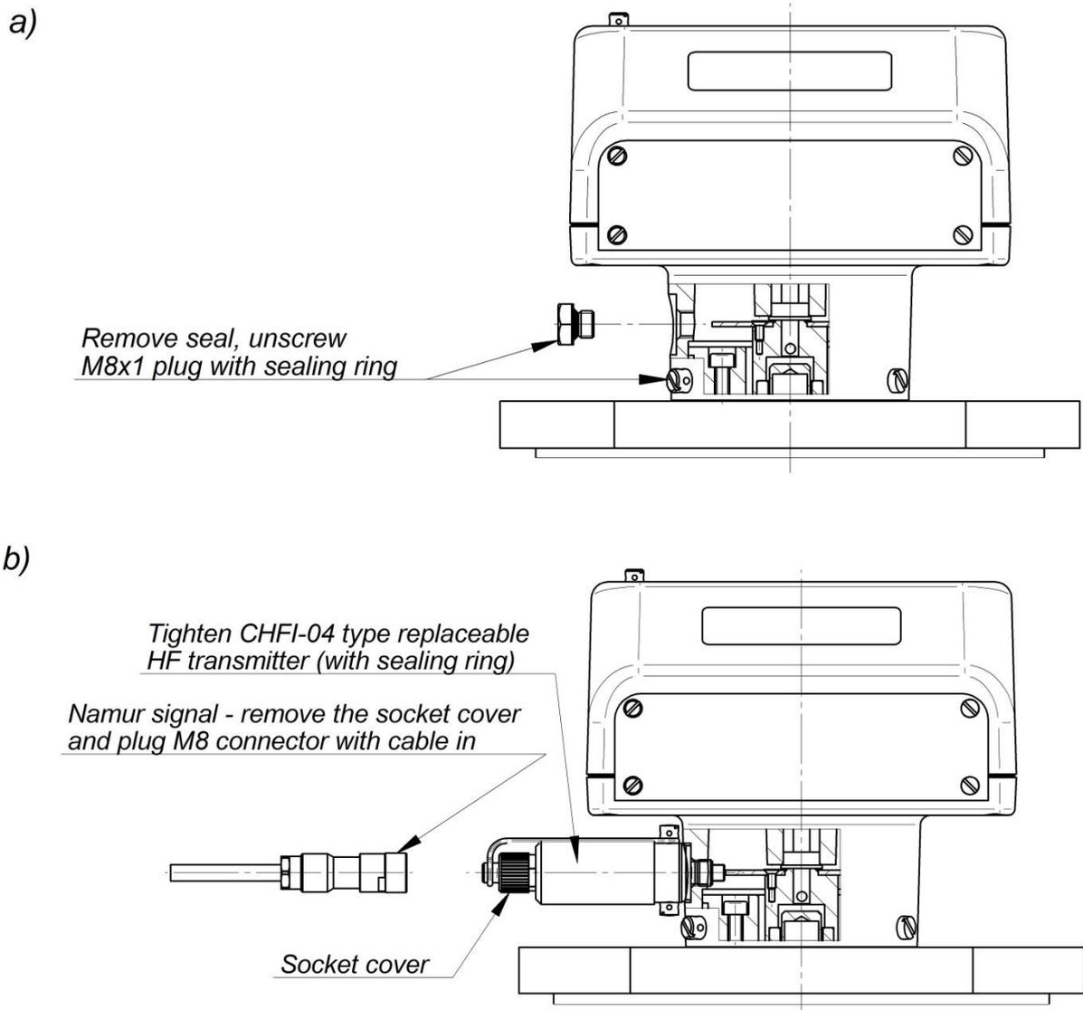
Fig. 17. Connection of the control element.
